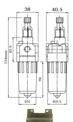
• Supply pressure 6 bar , pressure drop p=0.5 bar (for standard models)
